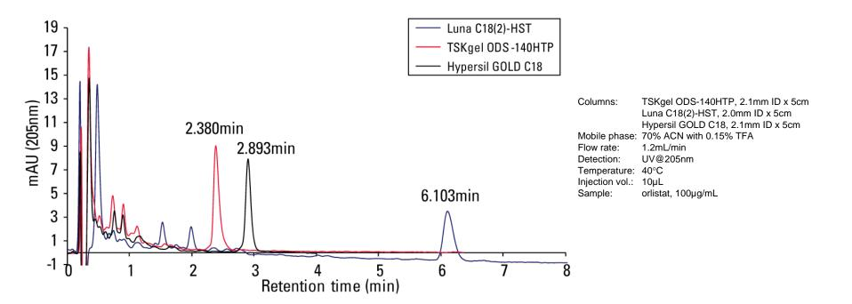
The TSKgel ODS-140HTP column yielded the shortest retention times in comparison to the other two competitive columns tested under identical chromatographic conditions.
